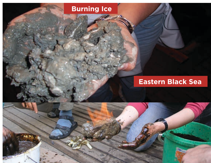
Figure 2. The 15 th (TTR, 2006) of UNESCO-supported Research and Training Voyages in the Black Sea, along with oil on the ship deck, the burning of GH sampled from the seafloor is seen. The photograph, which is taken by author's research team during the fieldwork, is shared by his courtesy.
